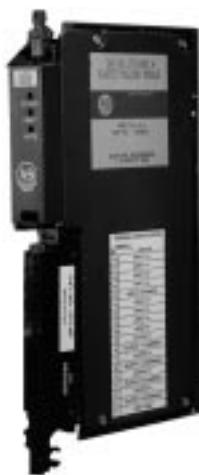
The Plastic Molding Module is a dedicated process module that controls the inject, clamp, and eject phases of an injection molding machine.
