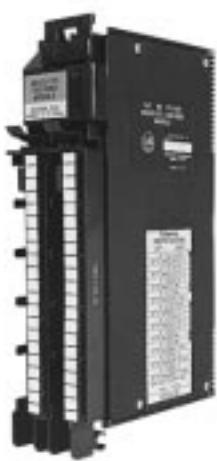
The Absolute Encoder Module converts a 12-bit (maximum) natural-binary or Gray-code value from an absolute encoder into a 16-bit (4-digit) BCD value. The module can also pass through a 12-bit (3-digit) BCD value from the encoder.
