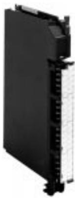
The 1771-VHSC is a single-slot module that contains four counters for encoders and provides one of the lowest costs-per-channel in the market. It features eight assignable high-current outputs and gives you the flexibility to assign any number of the eight outputs to a single counter.
