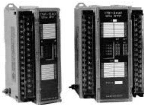
A 1791 I/O block is a compact unit that contains I/O circuits, a built-in power supply, and a remote I/O adapter. A 1791 I/O block is compatible with a remote I/O scanner of a PLC or SLC programmable controller when connected on an Allen-Bradley Universal Remote I/O link. The I/O values are accessible from the PLC or SLC data table.
