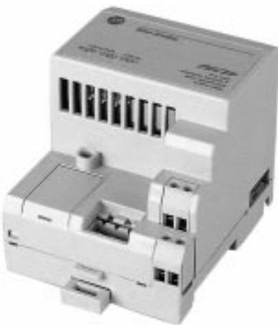
The 1794 remote FLEX I/O adapter module can interface FLEX I/O modules to a remote I/O scanner port of an SLC or PLC processor across a Universal Remote I/O link.
