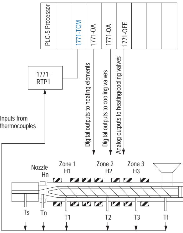
T = temperature measurement point (thermocouple)
