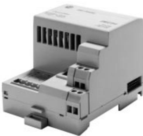
The DeviceNet FLEX I/O adapter module can interface 8 FLEX I/O modules (128 I/O devices *that are not DeviceNet-compatible*) to a DeviceNet scanner over a DeviceNet network. The DeviceNet FLEX I/O adapter lets you add many I/O devices to a system that has minimal PLC or SLC processor I/O image space available.
