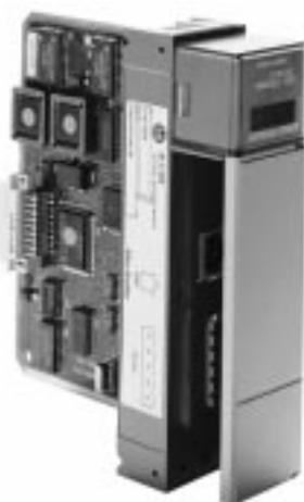
The SLC 500 DeviceNet scanner acts as an interface between DeviceNet devices and the SLC processor. The 1747-SDN is a single-slot I/O module that resides in the SLC modular chassis and provides a connection to one DeviceNet network. The scanner can communicate with 63 DeviceNet devices over the DeviceNet network to read inputs from a device, write outputs to a device, and monitor a device's operational status.
