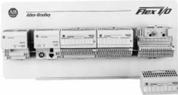
FLEX I/O provides a compact modular I/O assembly that consists of a maximum of 8 I/O modules, a terminal base for each I/O module, and an I/O adapter module with a built-in 24V-dc-input power supply. FLEX I/O can be used in PLC and SLC systems.
