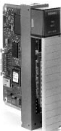
The 1746-QV Velocity Control Module is part of an SLC-based system for open-loop velocity control of a hydraulic ram. This intelligent I/O module receives velocity profiles from the SLC 500 processor. Profile set points define where to accelerate and decelerate for each new segment. The profile specifies the analog output to execute for each of 7 segments.
