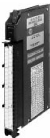
The 1771-CFM module interfaces PLC processors with magnetic pickups, single channel shaft encoders, turbine flowmeters, or any source of TTL pulses. The CFM module supports rates as high as 100kHz and counts as large as 9,999,999.
