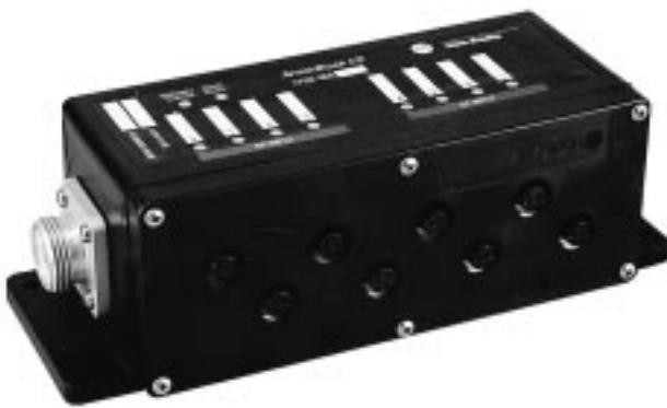
A 1792 ArmorBlock™ I/O block is a compact unit that contains I/O circuits, a built-in power supply, and a built-in DeviceNet I/O adapter. Because of its sealed housing, a 1792 I/O block requires no enclosure. It is compatible with a PLC or SLC programmable controller or other DeviceNet scanners. The I/O values are accessible from the PLC or SLC data table.
