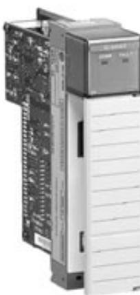
The SLC 500 Remote I/O Scanner enables communication between an SLC 5/02, 5/03, or 5/04 processor and remotely located operator interface and other adapter devices over the Universal Remote I/O link. The scanner can communicate with 1746 I/O, 1771 I/O, and 1794 I/O (FLEX I/O) modules and 1791 I/O blocks located up to 3048m (10,000 ft) away from the local SLC chassis.
