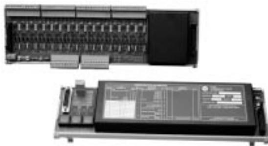
The Allen-Bradley Smart Transmitter (HART Protocol) Interface products let your PLC-5 family processors access all of the analog and digital information generated by your HART-compliant field devices (FDs). The digital process values can be used to qualify analog FD inputs, enabling your PLC-based programs to compensate more precisely and control your process more accurately.
