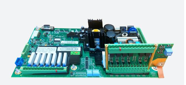
Control boards and capacitors are key components of AMVAC, R-MAG, and magnetically actuated Roll-in Replacement circuit breakers. Proper care, maintenance, and replacement of these components are essential to optimal reliability and operation.
