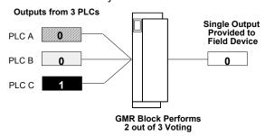
If only two of the three PLCs are communicating on the bus and they send matching output data for a point, the block group sets the output to that state.
