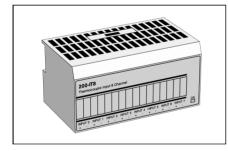
I/O unit for eight thermocouple input signals with programmable filters and 16-bit resolution. One bi-coloured LED indicates power on/off.
